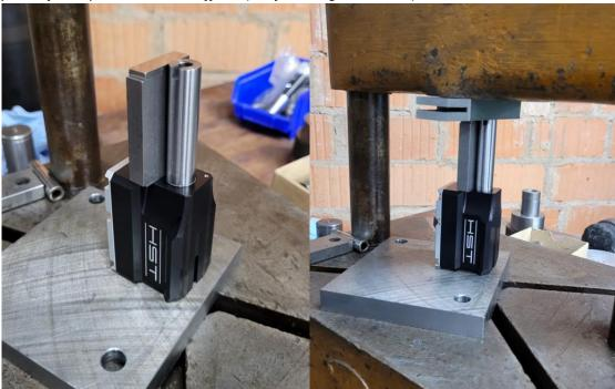
9. After pressing in, check the depth and alignment of the groove for the extractor. If necessary, press the barrel out again and install it again.
