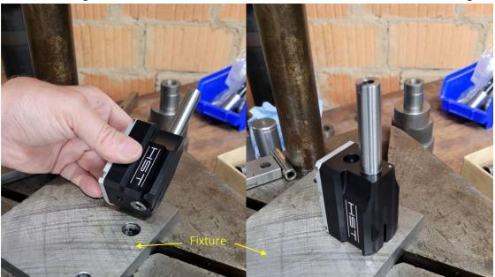
8. Press in the barrel according to the measured offset. The press-in depth was determined in the chapter 5.1 ("Removal"). **Be careful not to damage the barrel with tools!** *Hint: Build yourself a stop that limits the offsets (see following illustration).*
