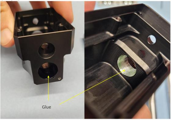
5. Put a slight amount of glue to the previously cleaned surfaces on the barrel. Use Loctite 638 (or equal).
